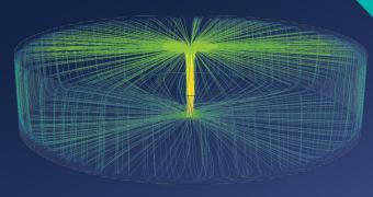
CFD modeling of a GridBee<sup>®</sup> GS Series Tank Mixer. Powerful mixing and large induced flow patterns such as this provide destratification and uniform water quality throughout the tank water column.
