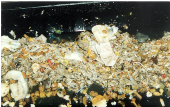
Fig. 4: Raw screenings in a sluice channel
