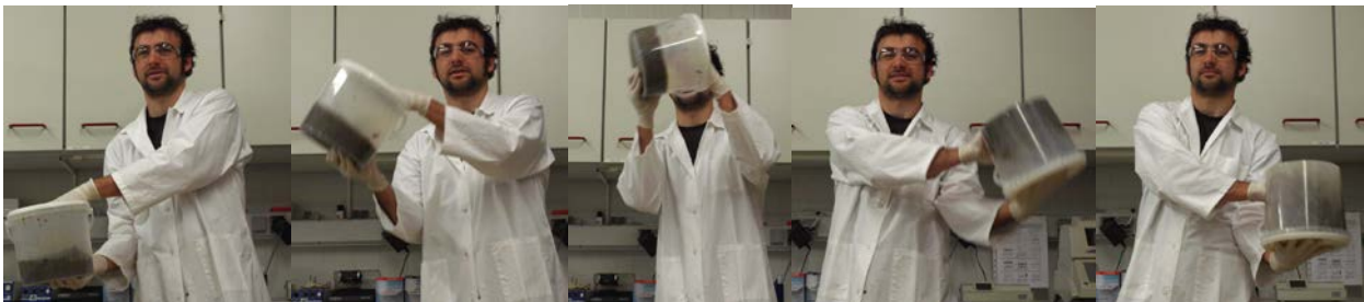
Figure 9: Manual tumbling method; the movement must be so quick that the liquid surface remains almost parallel to the buckets bottom (vertical) in its highest position
