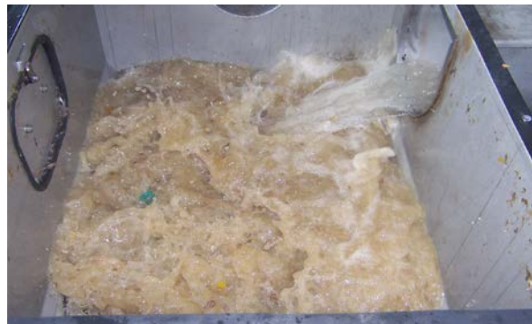
Fig. 5: High turbulence in the launder tank
