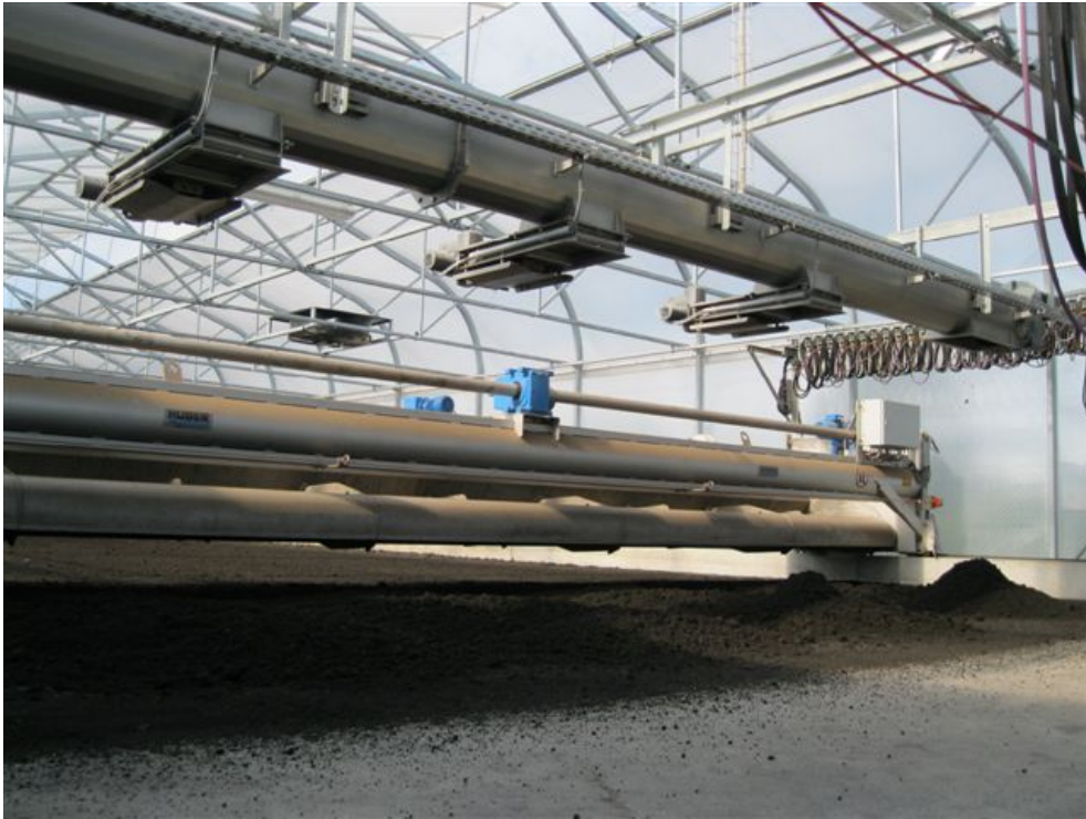
Figure 7: overhead screw conveyor design
