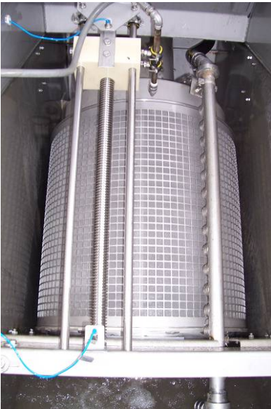
Figure 34 – Membrane Screen RoMEM with 0.5mm woven mesh
