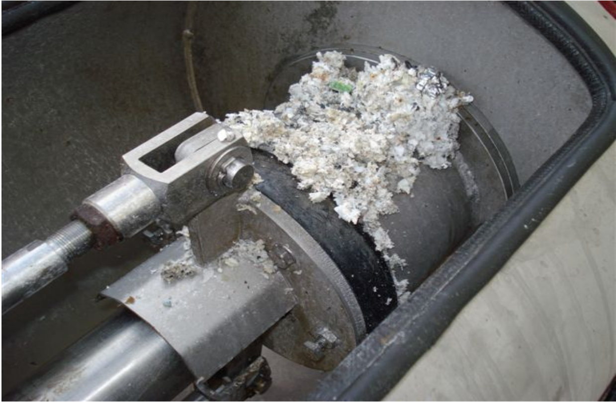
Paint chip removal with STRAINPRESS®
