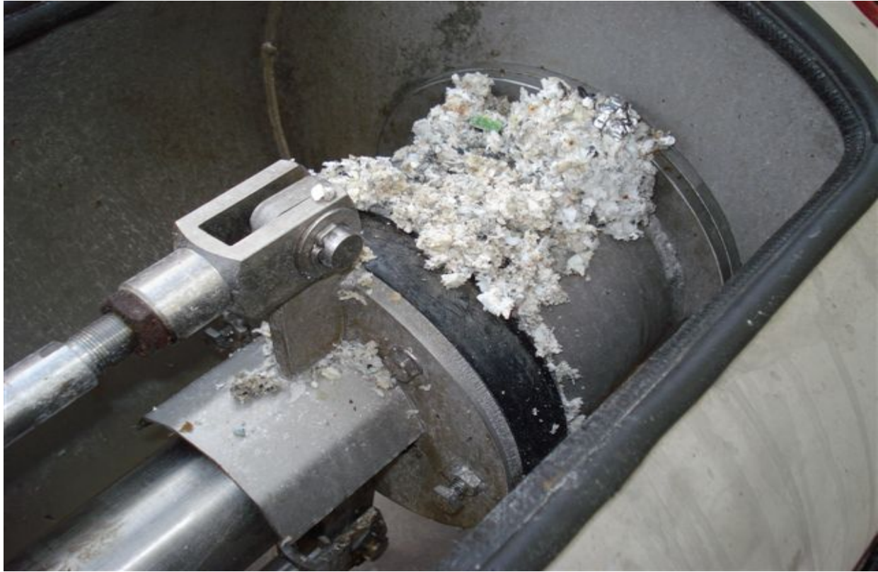
Paint chip removal with STRAINPRESS®
