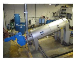
more effectively separates the water from the biosolids – practically creating a dryer solid end-product. The resulting water is cleaner than the water that comes into the headworks and produces no gaseous odor as it is fed back into the channel as the water does in the belt press process. This was critical for Bart in fulfilling his goal of improving the plant's impact on the community.
