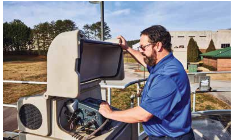
Fayard, shown with a Hach AS950 Autosampler, faces challenges that include increasingly strict permit limits.
