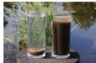
SV 10 comparison of aerobic granular sludge (left) and conventional activated sludge (right)
