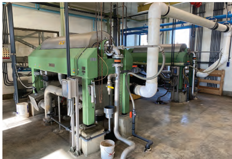
ABOVE: Two centrifuges (GEA Group) dewater biosolids delivered by newly installed Double Disc Pumps from Penn Valley Pump. LEFT: The Double Disc Pumps are designed for ease of maintenance with maintain-in-place hinged housings that enable quick disassembly and reassembly.
