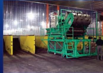
Agitated and Aerated In-vessel type Composting System (ICS)
