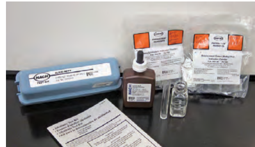
A portable alkalinity test kit (Hach) that uses powdered reagents and dilute sulfuric acid.
