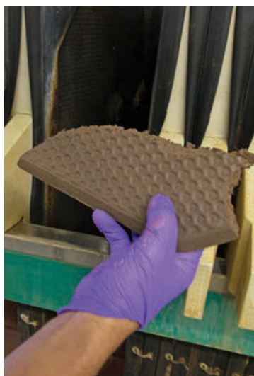
The facility's plate-and-frame press delivers high-quality biosolids cake.
