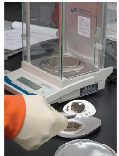
Mixed liquor suspended solids and return activated sludge samples are weighed on a balance (Denver Instrument).
