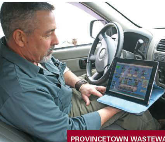
BELOW: Plant manager Chris Rowe uses an iPad to check the plant's SCADA system wirelessly. RIGHT: The Provincetown team includes, from left, operator Adam Curtis, plant manager Chris Rowe, operator Chris McKernan, and operator Reid Snow.
