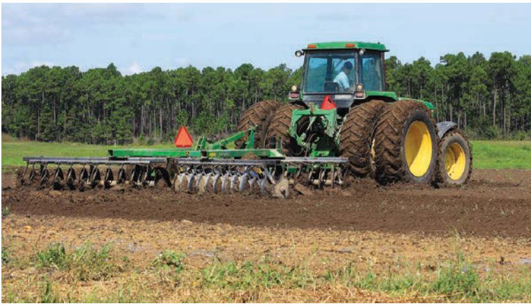
Operator Jesse Spear incorporates biosolids using a 15-foot John Deere disc harrow.
