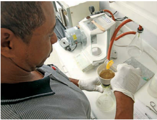
Plant supervisor Tim Thomas tests mixed liquor suspended solids.
