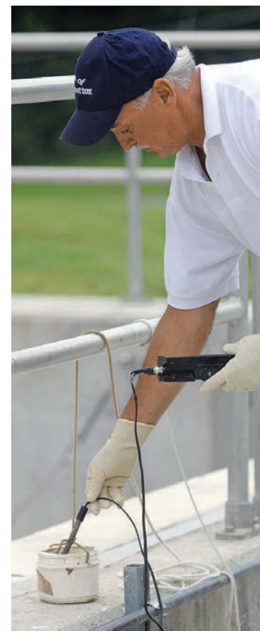
LEFT: From left, operators Patrick Witcher, Jerome Houston and Kyle Lerner and plant supervisor Mitch Stone check the water level of the reed beds used for biosolids treatment. BELOW: Stone checks the pH in a sequencing batch reactor basin. The plant team aims to maintain a pH of 7.8-7.9 to help with the zinc removal.
