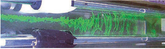
FIGURE 4. Vortex mixers add turbulence, ensuring that particles and microorganisms reach the UV lamps.
