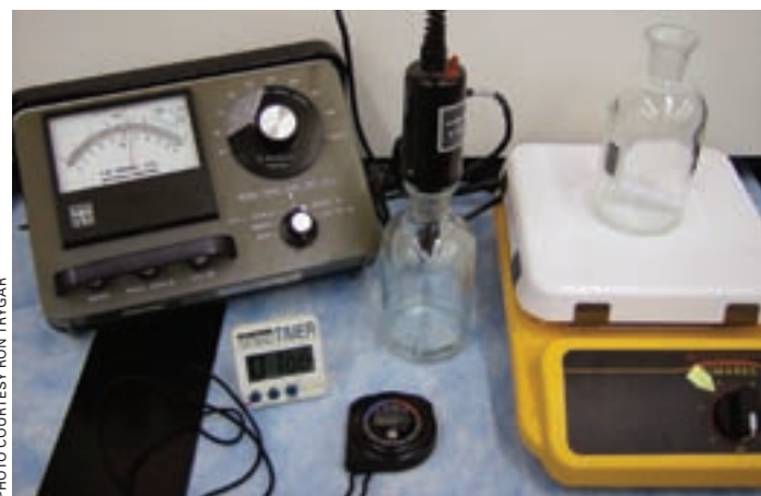
Examples of the tools used in oxygen update rate (OUR) testing include a YSI oxygen meter, timer, stopwatch, and a Barnstead/Thermolyne (Thermo Scientific) scale.
