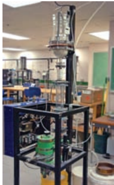
The University of Nevada – Reno’s prototype fluidized bed dryer was built in the chemical engineering lab. The university is now seeking partners and investors for a full-size commercial pilot project.
