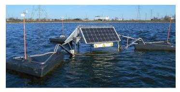
exit the pond much easier (as usually evidenced by up to 300 methane bubbles per square meter) across the entire lagoon. The increased methane release speeds up anaerobic digestion of bio-solids at the bottom. Better & more effective sludge reduction eliminates any need to ever dredge the ponds.
