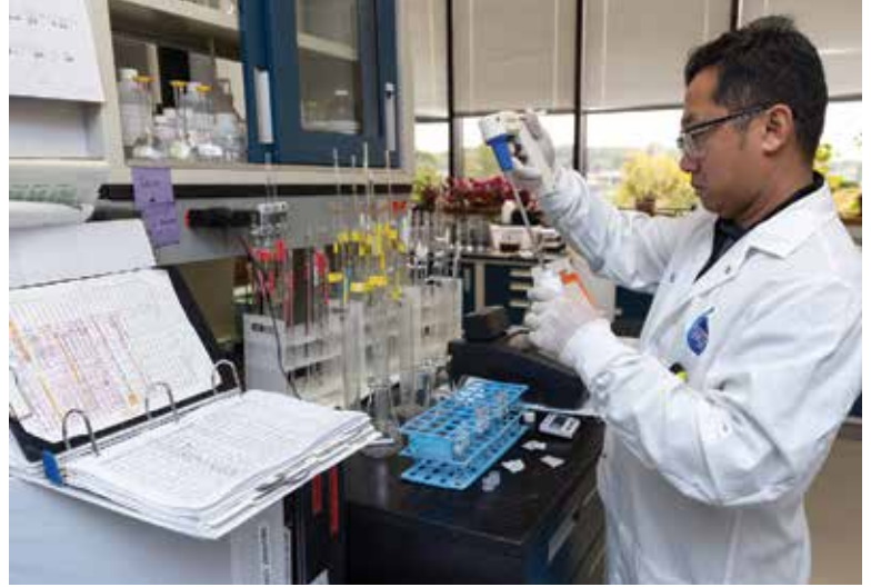
Quoc Chu, lab technician, runs a phosphorus test using a Hach DR2700 spectrophotometer and a Drummond Pipet-Aid portable pipette controller (Cole-Parmer).
