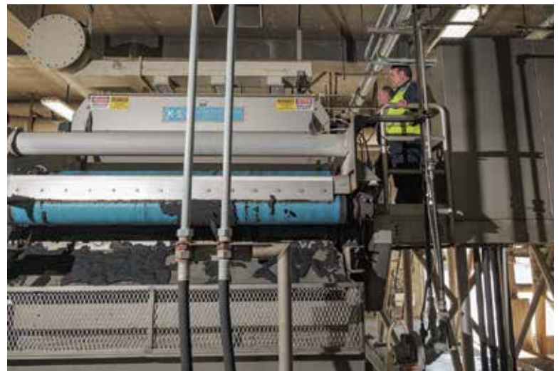
Quinn Miller and Dos Santos check on the Komline-Sanderson belt press.
