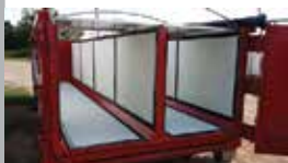
ADS dewatering unit from AQUA-Zyme Disposal Systems
