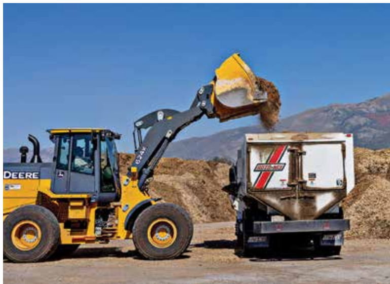
Wood chips are mixed with biosolids during the composting process (Roto-Mix twin-auger horizontal mixer).
