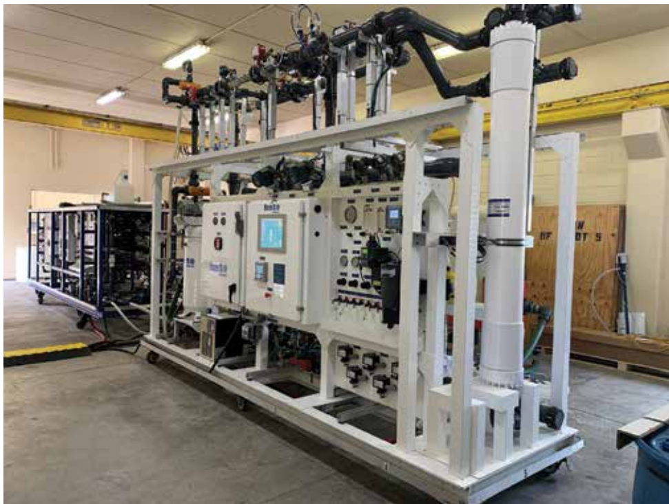
Microfiltration and reverse osmosis are among advanced treatment processes commonly deployed in direct potable reuse facilities.
