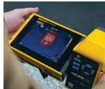
Thermal images are analyzed for hot spots that indicate issues needing attention (Fluke Corp.).
