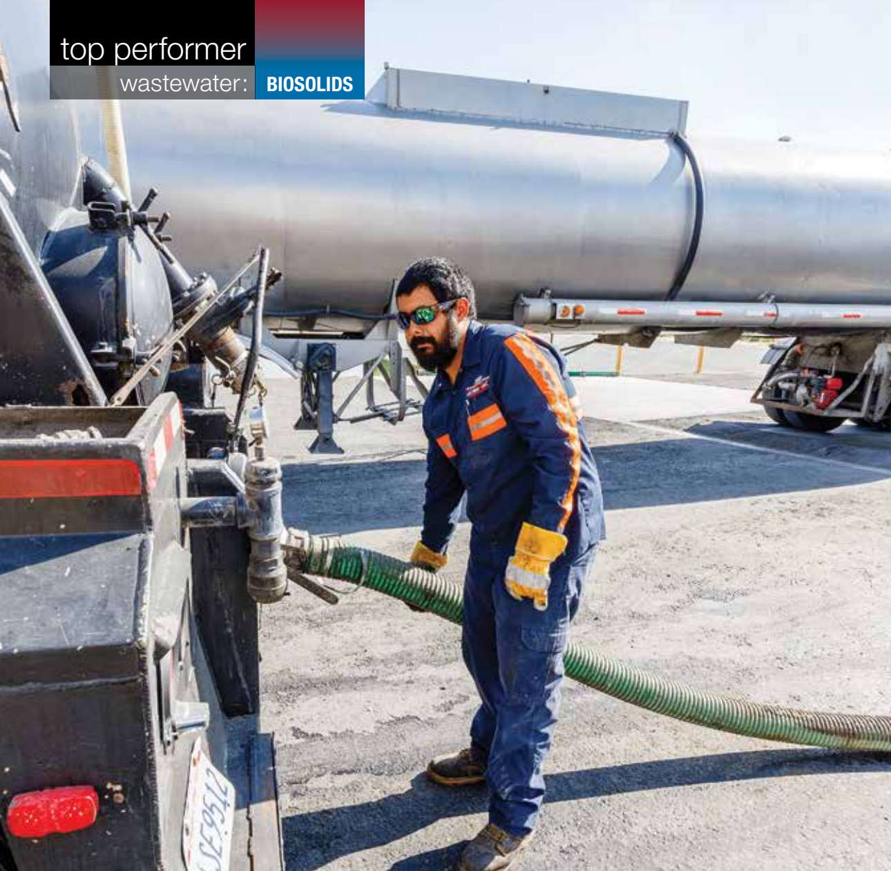
Truck driver Jose Garcia offloads industrial food waste (leftovers from beer and fruit juice making) at the Victor Valley Wastewater Reclamation Authority's biogas production facility.
