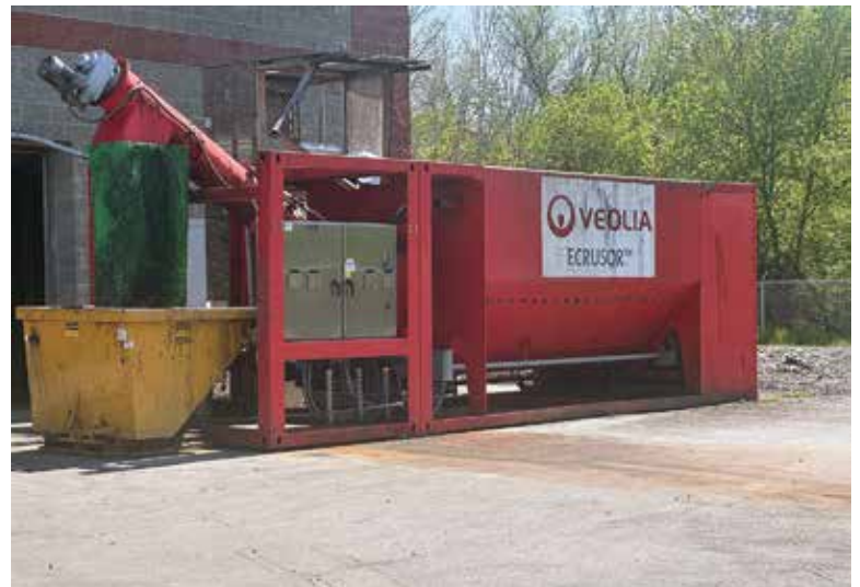
The eCrusor (Veolia Water Technologies) de-packages food in plastic jars without shattering the brittle plastic lids.
