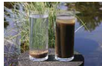
SVI 30 comparison of aerobic granular sludge (left) and conventional activated sludge (right)
