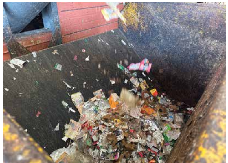
The Turbo Separator removes food products from the packaging and spits the waste material into a hopper.
