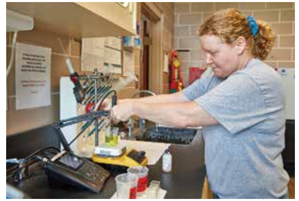
Fowler checks the source water using an Orion Star A211 pH meter and Cimarec digital stirrer from Thermo Fisher Scientific.
