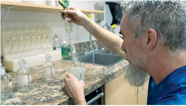
Peterson pipettes a sample to a BOD test bottle.
