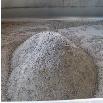
The cleaning process yields washed street sweepings that can be reused.
