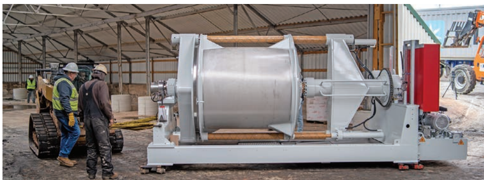
The Bucher filter press, shown being moved into the wastewater treatment plant, will dry biosolids processed by hydrothermal carbonization to 50-60% solids.
