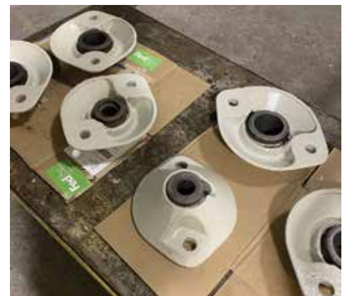
Graphalloy bearings in housings awaiting installation.
