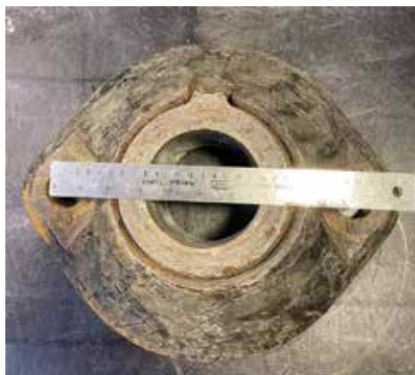
The original Babbitt bearing in its housing. This was later replaced with a Graphalloy bearing.
