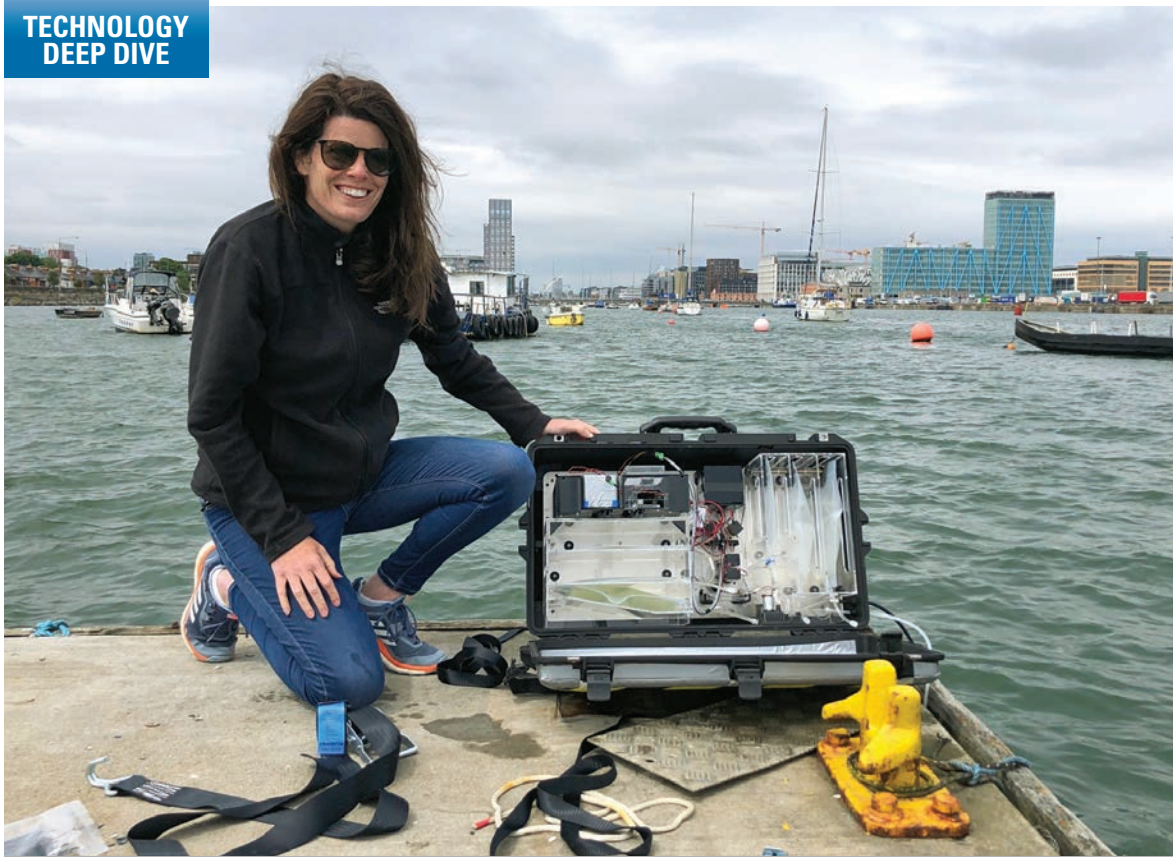
The PO4 phosphate sensor takes samples at different depths and uses a colorimetric method to measure the concentration. It can be mounted on LG Sonic's legacy buoys at strategic locations in a water reservoir.
