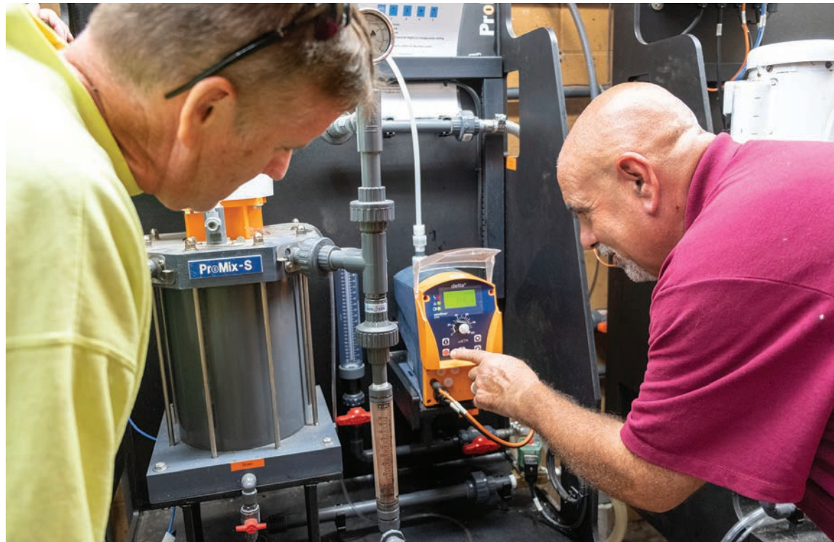
After reviewing recent testing results, Bill McCue (left) and Daniel Wurst make adjustments to the ProMix-S polymer mixing system (ProMinent Fluid Controls).
