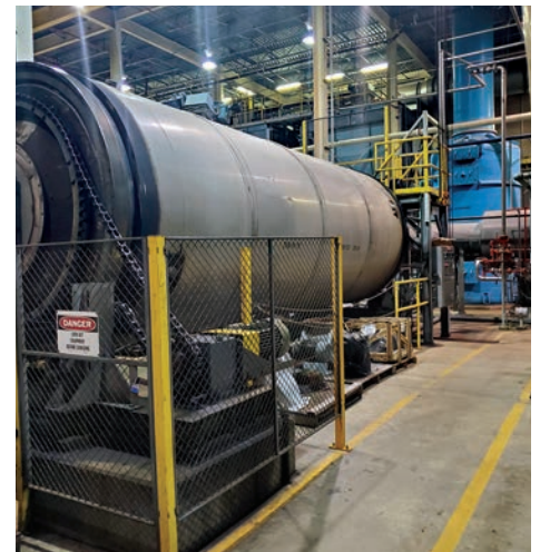
The final drying stage for Class A biosolids production is this rotary drum dryer (Baker-Rullman).
