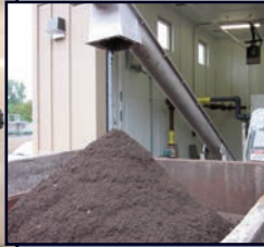
Discharge Cake from BDP Screw Press
