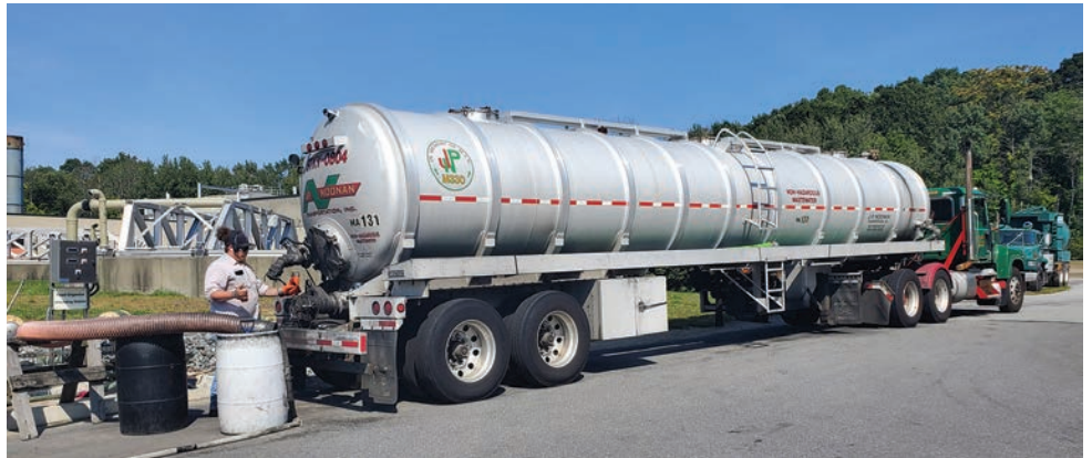
Food waste slurry is delivered to the wastewater treatment plant in tanker trucks.
