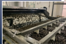
Independent Gravity Zone of 3DP Belt Press
