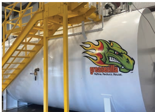
The Greasezilla unit removes FOG from the grease trap waste stream, reducing disposal costs and creating a new revenue source.
