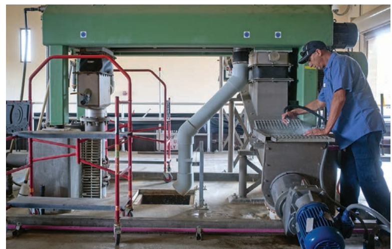
Schroeder cleans the centrifuge (GEA Group) at the Jomax facility.
