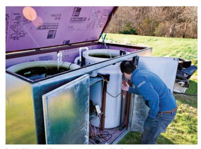
Brady O'Leary of Triplepoint prepared the NitrOx system for pilot testing.
