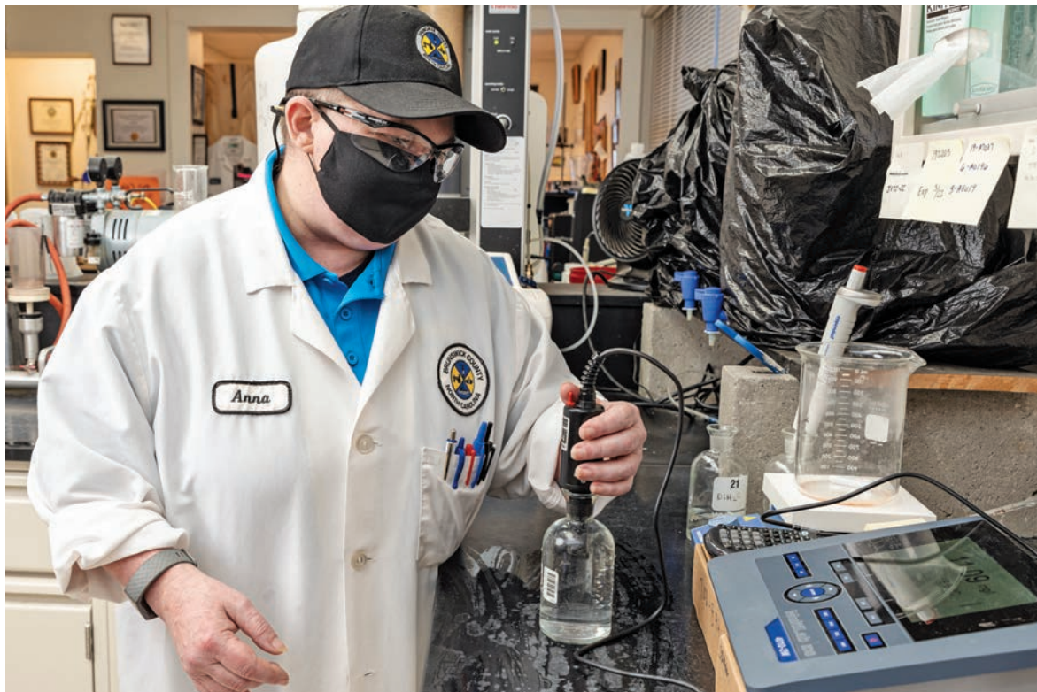
Anna leRoux (right) and Dana Nelson run samples on a Hach DR3900 spectrophotometer.
