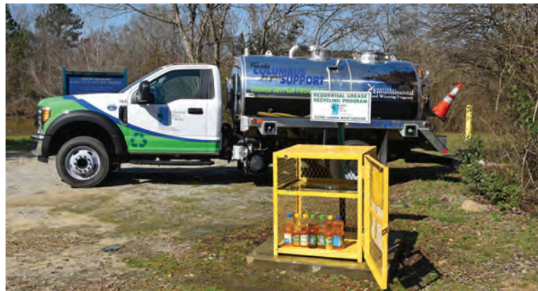
A Columbus Water Works truck collects grease that is added to the digesters to boost methane production.
