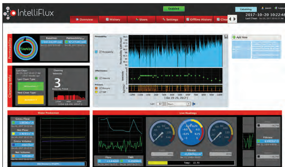
The reporting tool is customized for every facility by the design engineer and the plant operations team to report the plant's response to changing influent quality.
