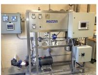
**injection system** with pipeline flash reactor provided the ozone mass transfer needed to remove color and odor while minimizing bromates.
