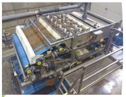
**Bright Technologies** offers complete **Belt Filter Press** dewatering systems that are skid or trailer mounted. We design and manufacture the skid equipment package for high throughput, low maintenance, superior cake solids and ease of operation.
