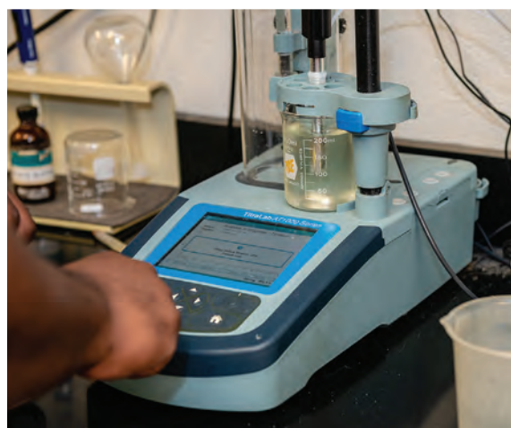
A titration analysis is taken using a Hach TitraLab AT1000. Titration and pH are the routine tests performed at the Duck Creek facility.
