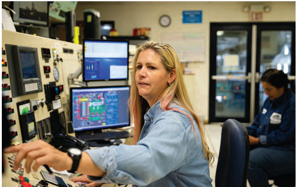
ABOVE: Michelle Tarantino checks the control panel for one of the facility's gas-fueled furnaces. It uses either natural gas or methane piped in from a nearby landfill. BELOW: Tarantino takes a sample of the dewatered biosolids before the material is fed into the furnace.
