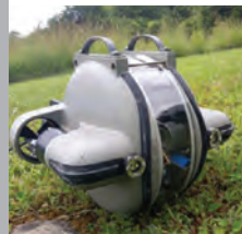
Potable tanks inspections from Pittsburg Tank & Tower Group
