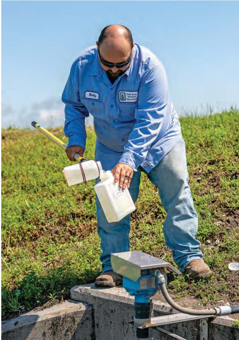
Bobby Reeves, maintenance worker and facility safety representative, collects a water sample from a wetland cell. Samples are collected weekly and sent to the Wylie Water Treatment Plant for testing.
