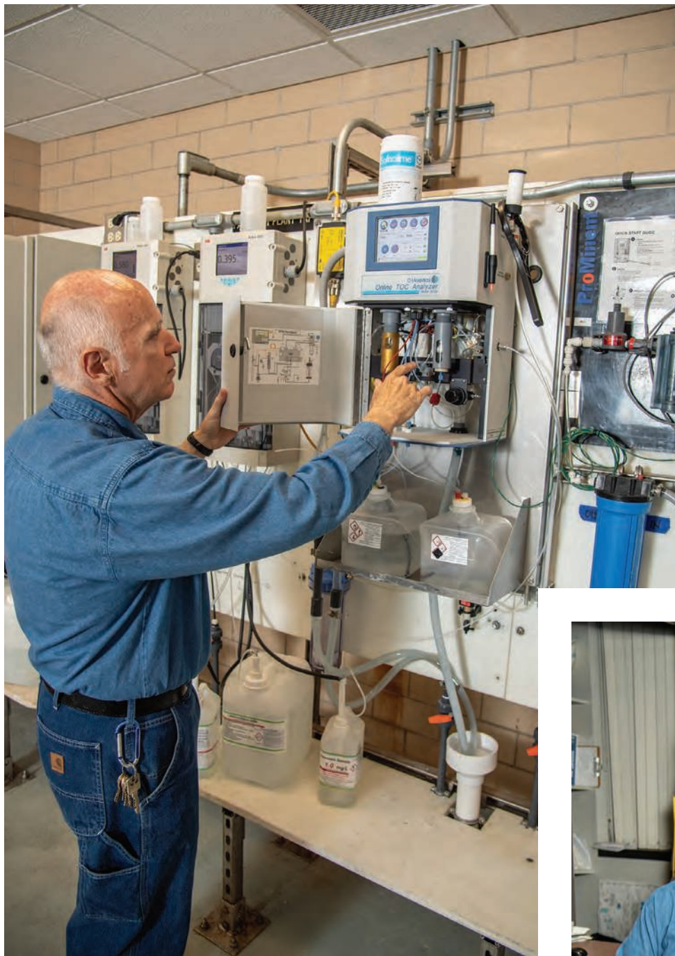
Joe Cribbs checks the 9210p Online TOC Analyzer (OI Analytical, a xylem brand) in the Tap 1 analyzer room.
