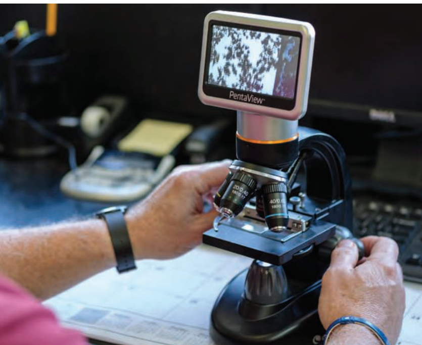
A lab technician reviews bacteria counts using a PentaView digital microscope (Celestron).
