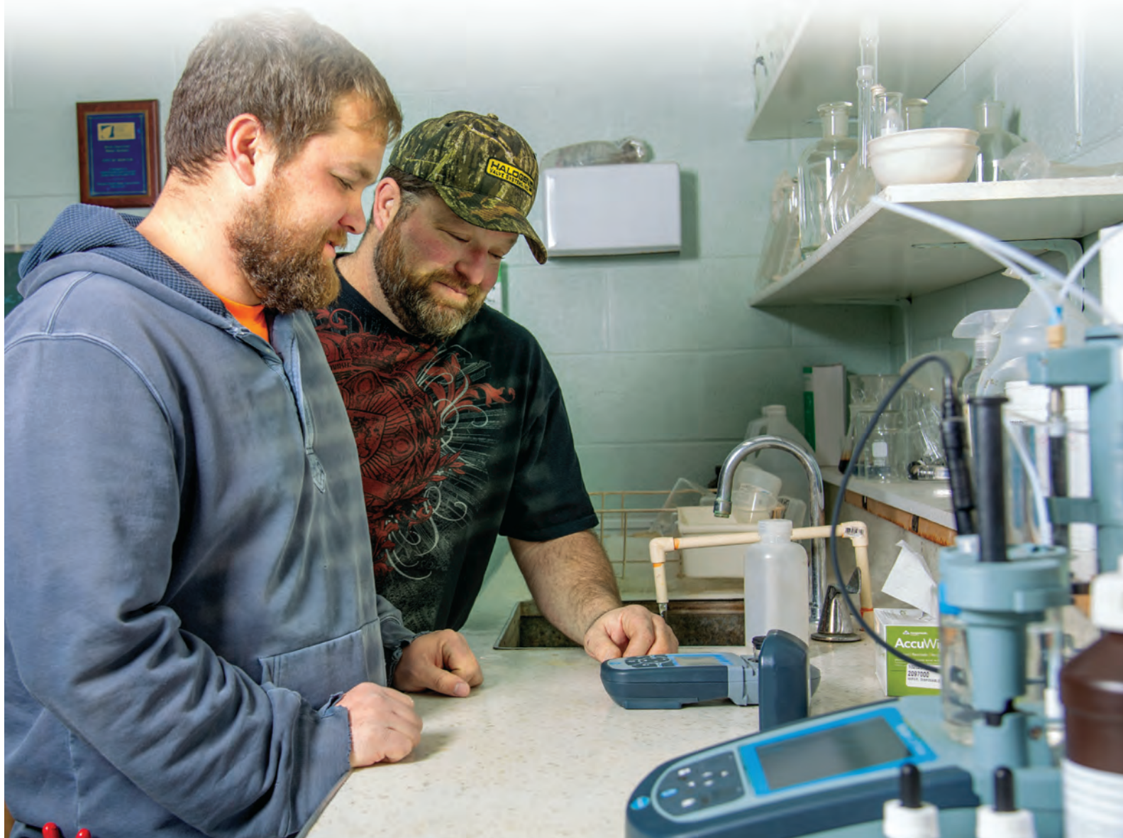
Norton Water Treatment Plant supervisor Jamie Amlong (left), and operator Drew Eagleburger check water turbidity using a Hach 2100N turbidimeter.
