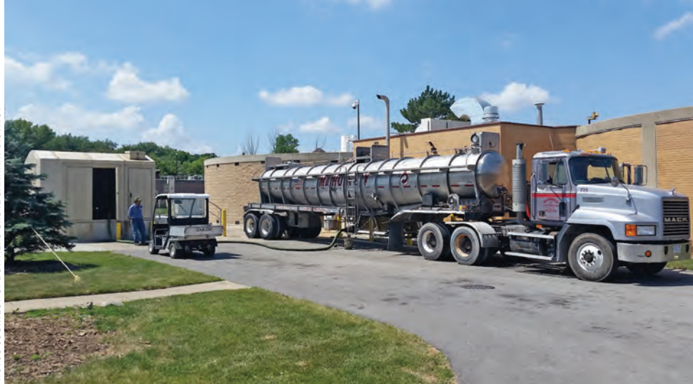
A contractor delivers a tanker load of grease to the Downers Grove (Illinois) receiving station. The grease will be fed to the anaerobic digesters.
