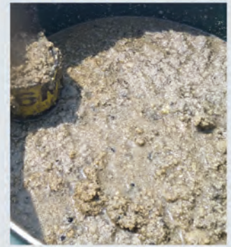
Coagulated grease with the consistency of oatmeal.
