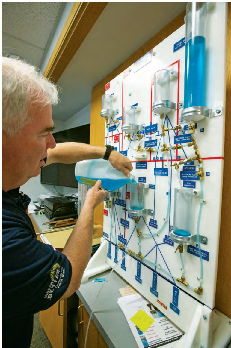
Randy Randall, with a water system model showing how to use gravity or existing pressure to push water through the distribution system without using energy.
