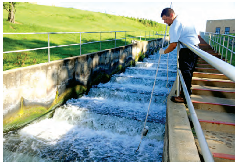
Jacob Oney, water reclamation operator, samples the outfall at Prince William County’s H.L. Mooney Advanced Water Reclamation Facility.
