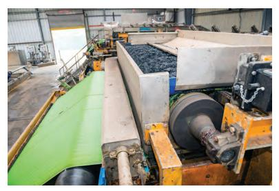
Biosolids are moved through a belt filter press at the Renda facility (Andritz Separation).
