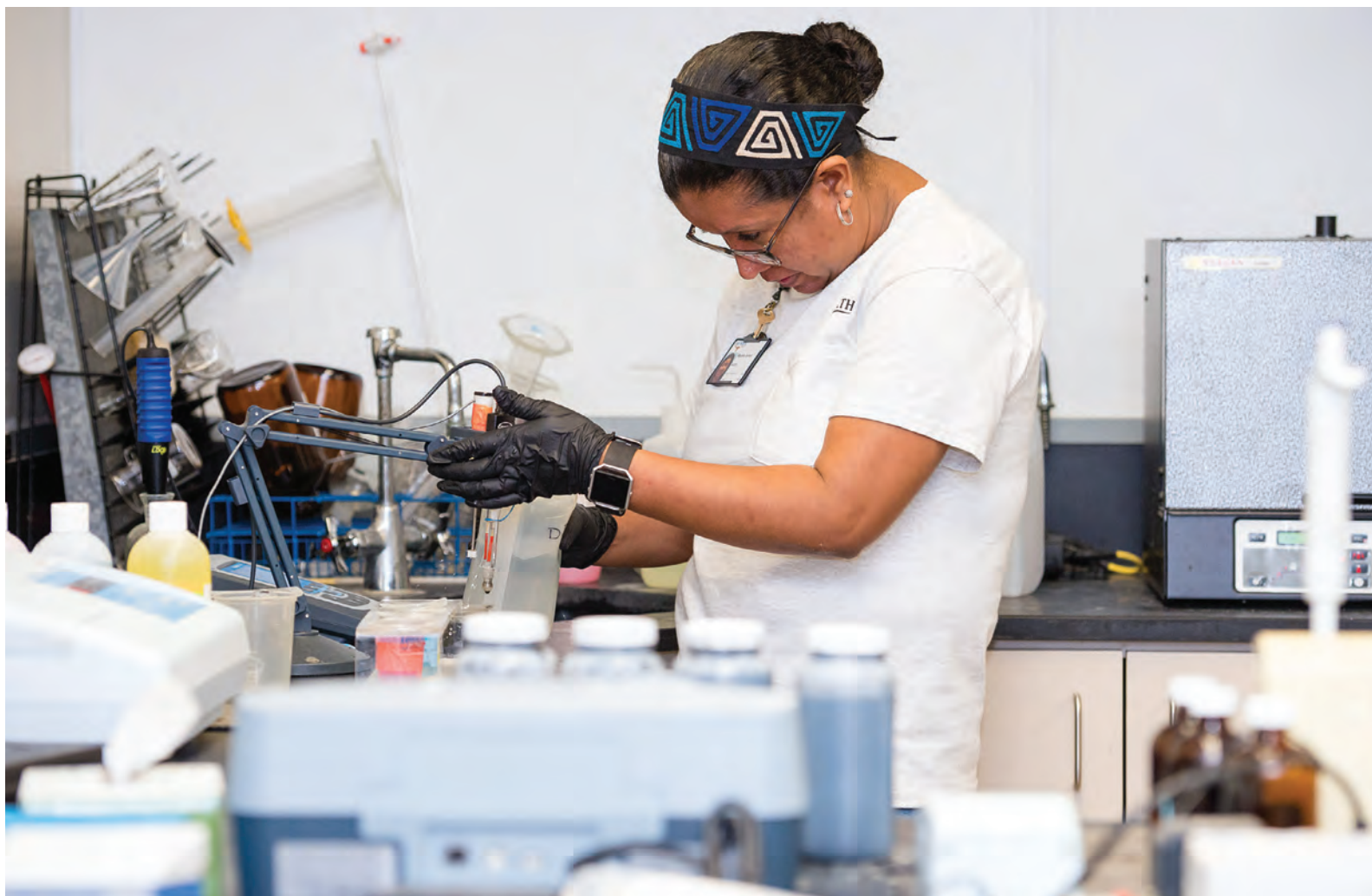
Migdalia Jackson, environmental specialist, works in the on-site laboratory testing samples for a pilot program for automatic odor control in the gravity thickener area. She prepares to use an OdaLog (Thermo Fisher Scientific) to test for hydrogen sulfide levels.
