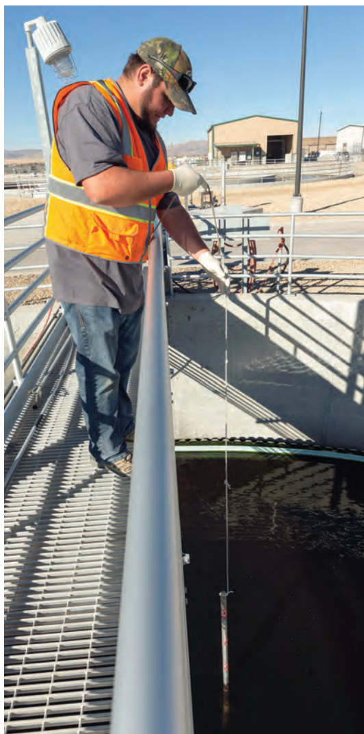
Brody Kinder uses a Sludge Judge sampler (Nasco) to measure the clarifier sludge blanket.
