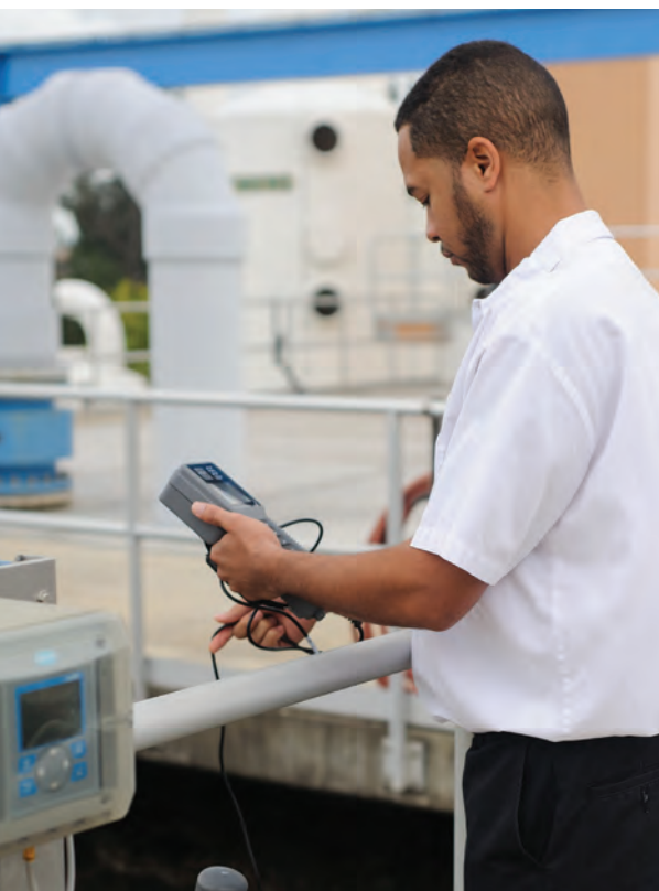
Walter Fletcher, plant operator 1, checks plant readings using a Model 55 dissolved oxygen meter (YSI, a Xylem brand).
