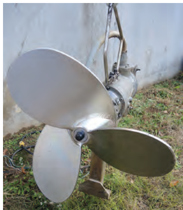
The Durham County team chose mixers with stainless steel impeller blades for extended service life.
