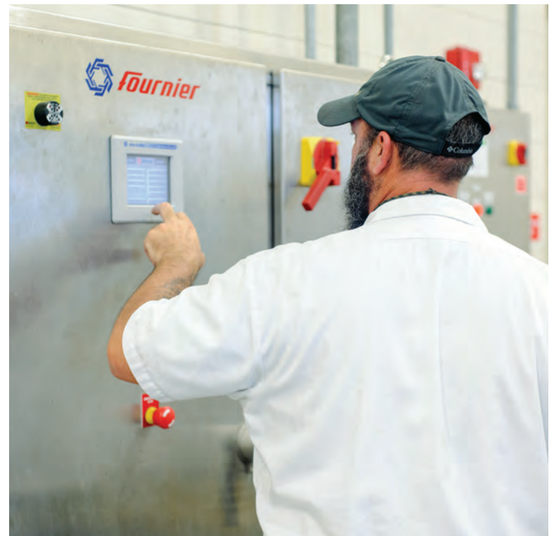
Todd Tysinger checks settings for the rotary press (Fournier Industries) used to dewater solids before transport to farms for land application.
