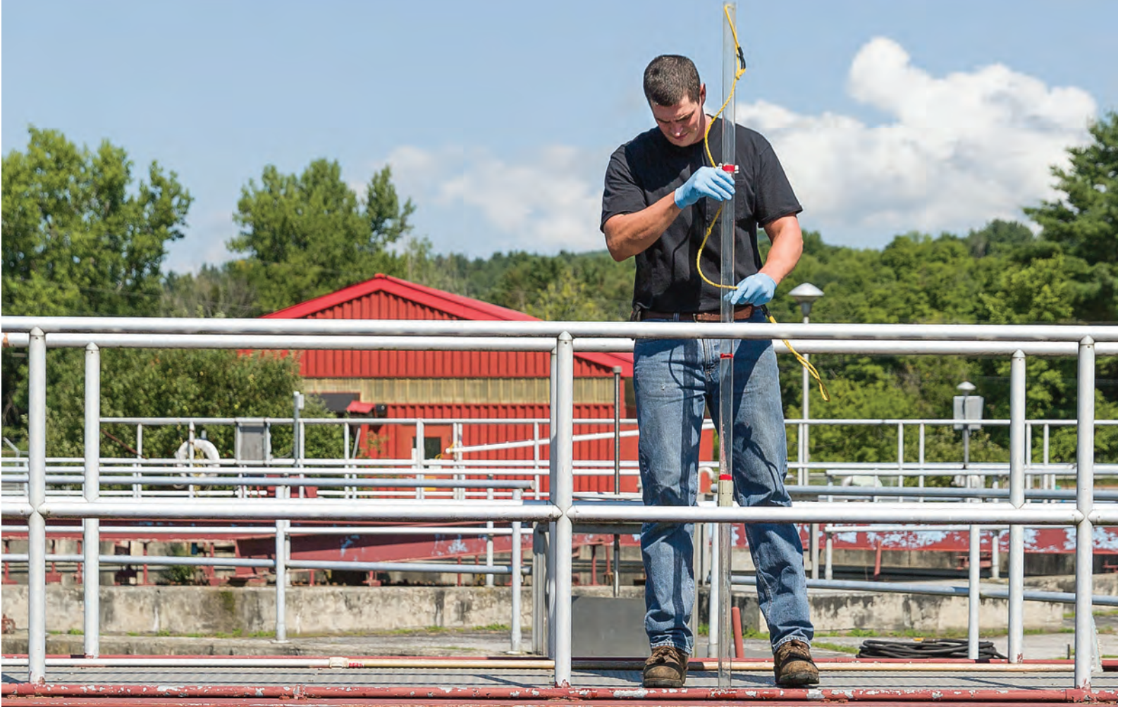
Cox uses a Sludge Judge (Nasco) to measure a sludge blanket.
