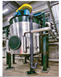
Thermal Hydrolysis System from Lystek International
