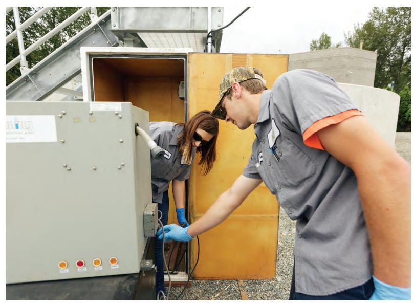
ABOVE: Matt Ellingson (right) and Danielle Lee reattach a sample controller (Manning Environmental) to a replacement refrigerator used as a composite sampler. BELOW: Clay Watkins checks dewatered cake from a centrifuge in a Fenton biosolids dryer (RDP Technologies).
