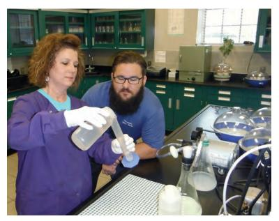
Missy Rhoades, lab manager, and Tyler Perdue test for TSS in effluent. Despite shutting down one aeration basin and reducing energy use for aeration in the other basin, the plant achieves 99 percent TSS reduction and easily meets its permit. about six hours apiece per day, and a pair of 40 hp mixers operating 11 hours per day. To save energy needs, the EMI suggested shutting down one basin and operating the other anoxically for about six hours per day.
