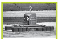
Surplus coarse bubble mechanical self-aspirating aerators and mixers, 30hp design. \$5,000 each. Refurbished 1-year warranty. Versatile installation, durable and simple to maintain. Motors not included.
